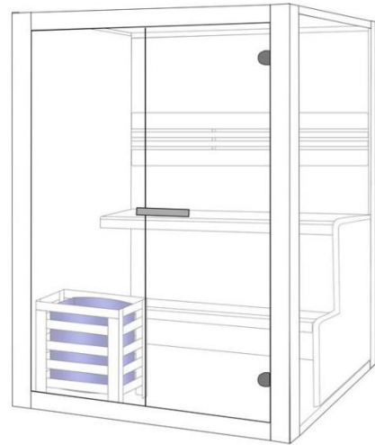
(13) Install sauna oven on the fence according to oven manual.
