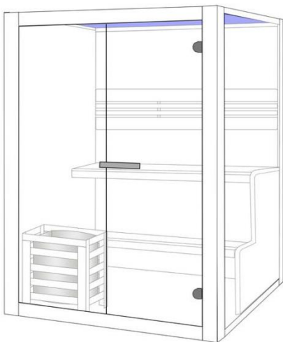
(14) Place Ceiling panel on the installed panels
